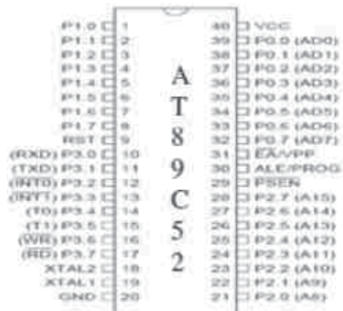
Fig.7: Pin details of AT89C52
